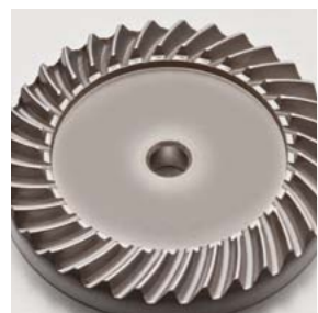
Shaping of complex parts. The example shows a crown wheel with a involute tooth geometry.
