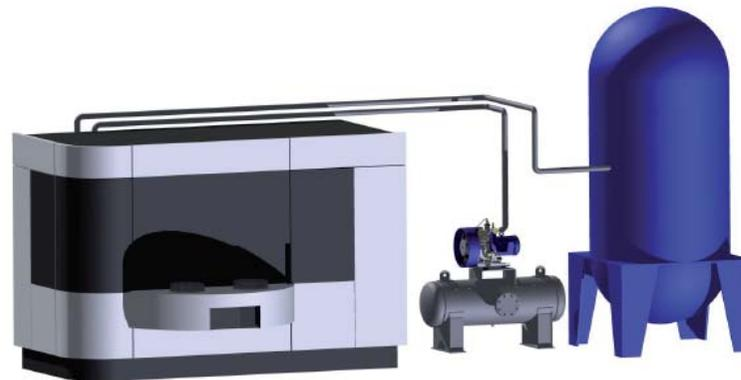
Version 3: Natural gas compressor and oxygen tank
