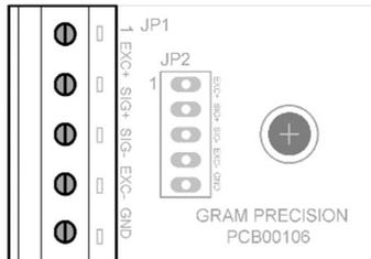
The cell cable is connected in the “JP1” power strip according to indications in the following table:
