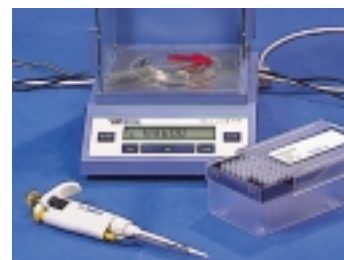
4. weigh the filled capillary with holding device and register the value. That's it.
