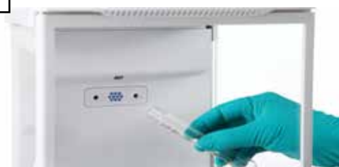
Built-in ionizer neutralizes static charges
