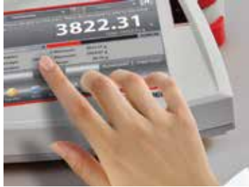
Resistive touch screen display quickly responds to operator's touch
