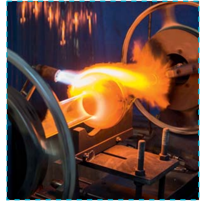
Glass tubes are blown by highly skilled blowers to ensure the excellent quality.
