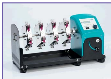
Rotisserie accesory for 1,5 ml centrifuge tubes hold horizontally.
