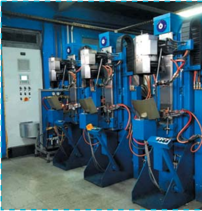
State-of-art, automatic welding machines are used to connect the foot to the cylinder.
