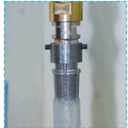
Grinding process of all joints performed by diamond reamers for best results.
