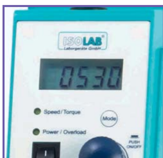
Large LCD display panel for indication of actual speed.
