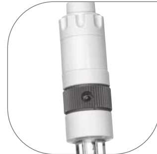
Twist-open the cap to expose the refilling hole
