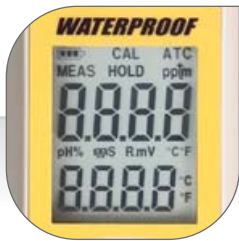
Large custom dual-display LCD
