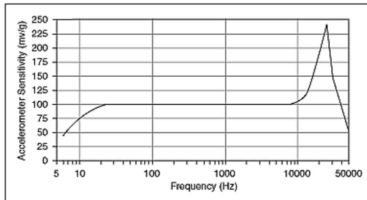
Figure 5 - Accelerometers sensitivity vs. frequency
