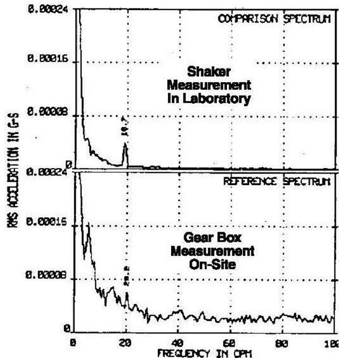
Figure 8 - Comparison spectra of laboratory vs. on-site measurements
