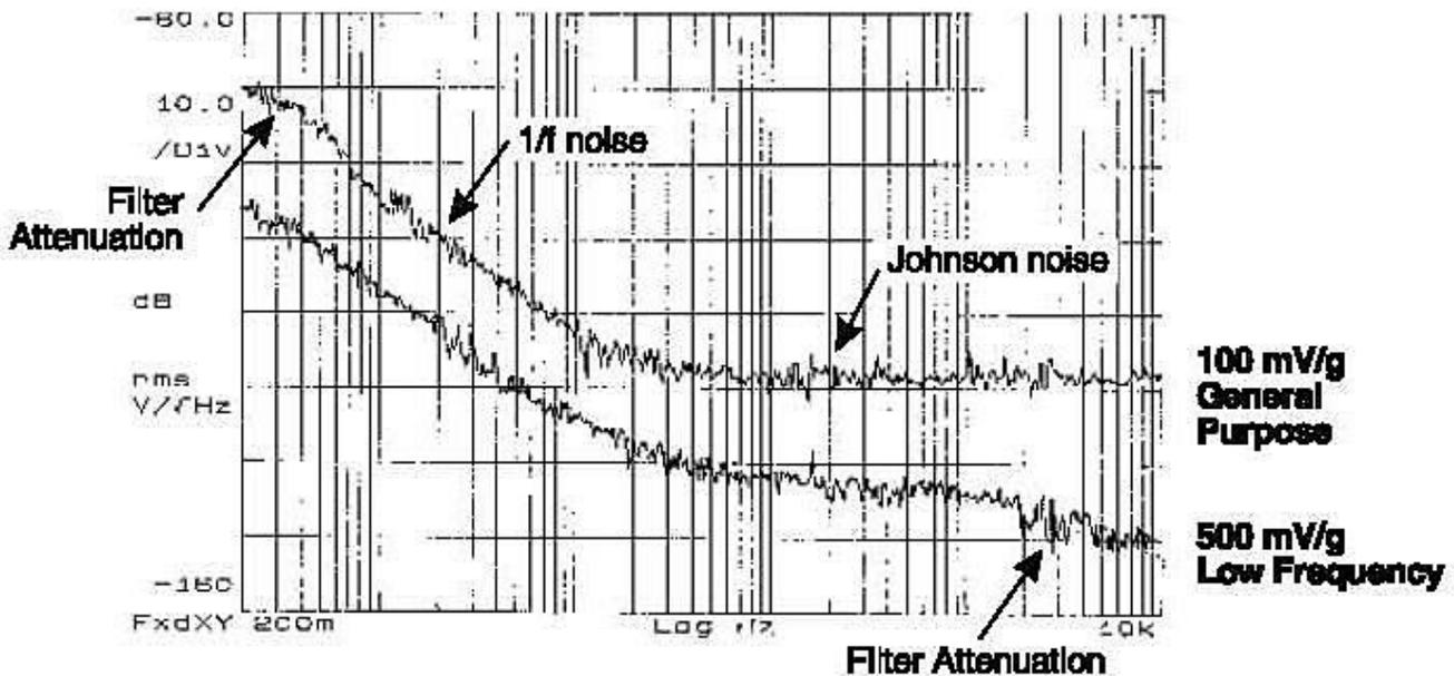
Figure 6 - Noise plot of 100 mV/g and 500 mV/g sensors
