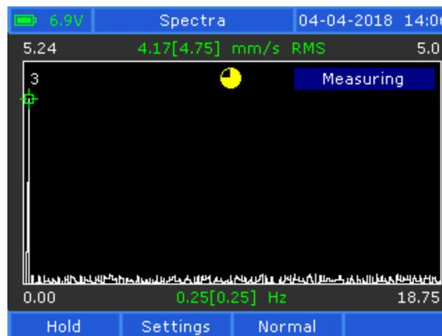
The measurements can be done with standard accelerometers, but better results can be obtained with high sensitivity accelerometers (500 mV/g).
