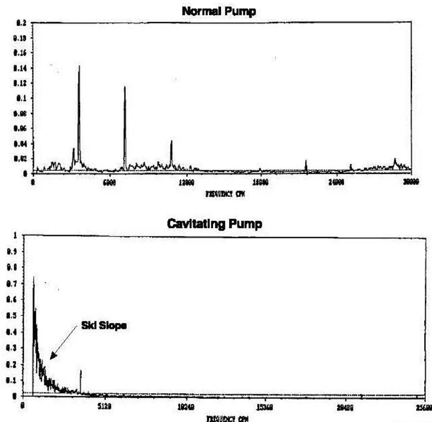
*Figure 7 - Low frequency signal overloaded from high frequency pump cavitation*
