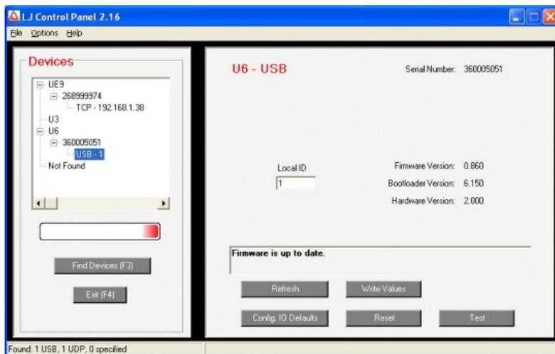
Figure 1.1-1. LJControlPanel Device Window
