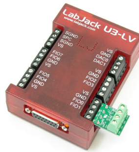
Figure 2: LJTick-VRef-25 with U3-LV
