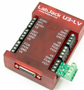
Figure 4: LJTick-VRef-41 with U3-LV
