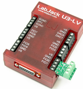
Figure 2: LJTICK-DigitalOut5V with U3-LV
