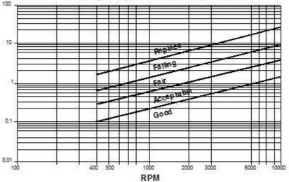
The diagram above is only a guide to interpret the Bearing Energy value. If vibrations of other causes (flow surge, gear mesh) are within in the frequency range 2200-20000 Hz, this can give a high bearing condition value without the bearing being damaged.
