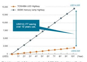
[Calculation condition] O Annual operation time: 3,000h Number of fixture: 10 units O Rate of electric utility: USD 0.11/kWh
