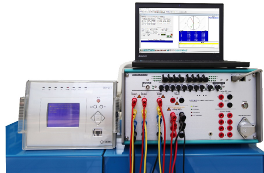
PW636i-F test traditional protective relay (Analog + Binary)
