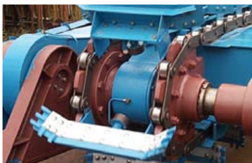
Reclaimer boom with double strand conveyor chain and bucket guiding rollers.
