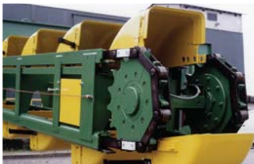
Boom of a bucket reclaimer with double strand conveyor chain.
