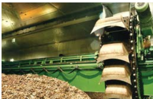
Bucket reclaimer in a biomass stockyard.
