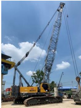
Crawler Crane 100 T
