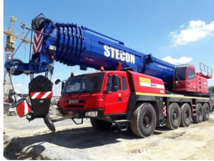
All Terrain Crane 220 T
