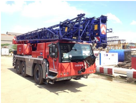
All Terrain Crane 60 T
