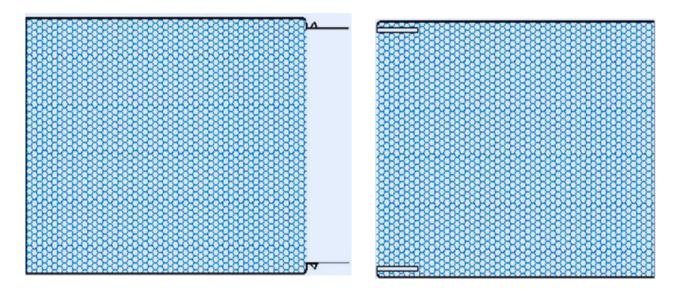
All panels utilize a cam-lock joint system with interlocking steel edges and internal locking hooks spaced every 20 cm along the length, ensuring an airtight, secure fit.
