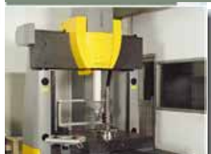
German ZEISS three-coordinate measuring machine
