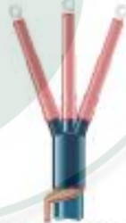
Heat-shrink termination, 3c paper MIND
