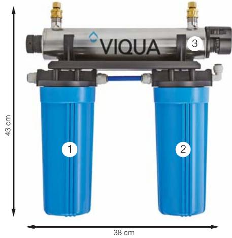
This compact multi point system allows for simple installation and operation. It is equipped with a **10" 5 micron sediment filter (1)**, removes dirt. A **10" carbon filter (2)**, removes taste and odour of chlorine. A **17 W** high output UV light which kills 99.99% of bacteria and viruses, encased in a **stainless steel UV chamber (3)**. Maximum water pressure 6.9 Bar.
