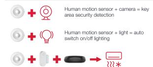
Human motion + door sensor + universal remote control = air conditioner-home/leave mode: automatic switching device
