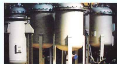
Mother batch tank/filtrate tank
