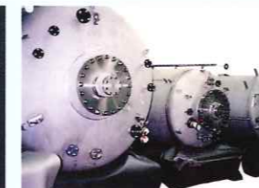
High-purity chemicals supply tank
