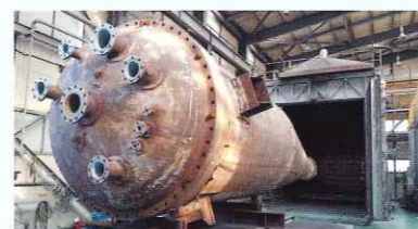
Low Pressure Separator
