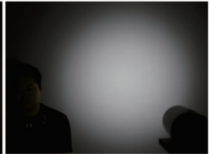
Test result of lens anti-glare louvre
