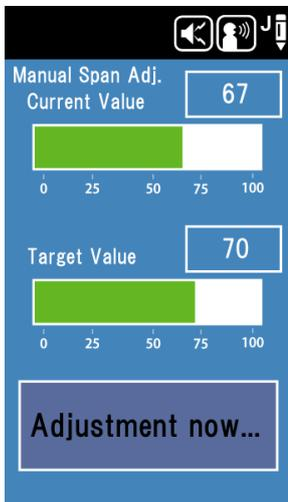
A successfully completed span adjustment displays the following screen.
