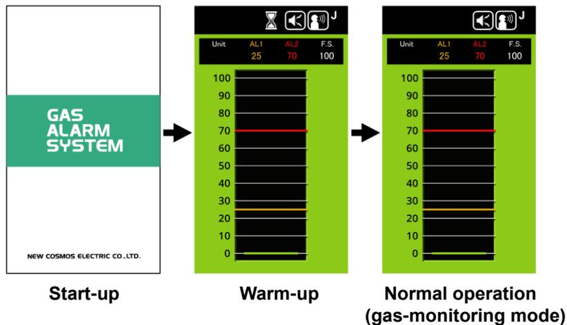
\*These drawings are just for an example. The screen differs depending on the delivery specifications.
