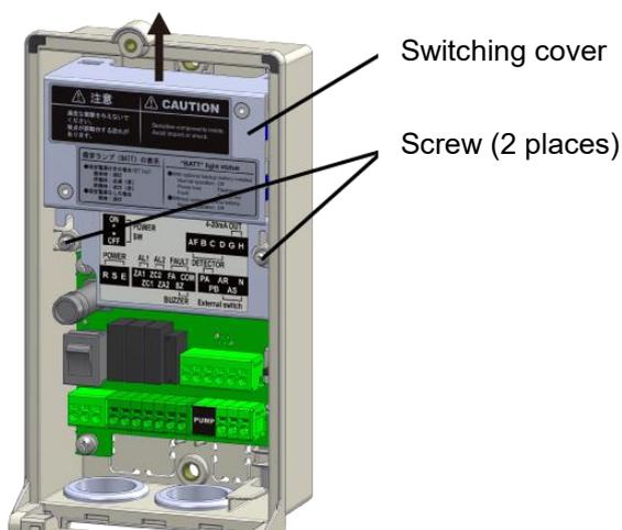
**4 Disconnect the two connectors from the AC-DC power supply unit. Detach the switching cover from the unit.**
