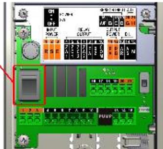
**3 Loosen the two screws. Slide the switching cover up.**
