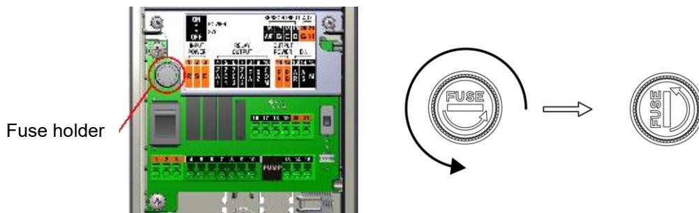
**4 Replace the fuse with a new one.**
