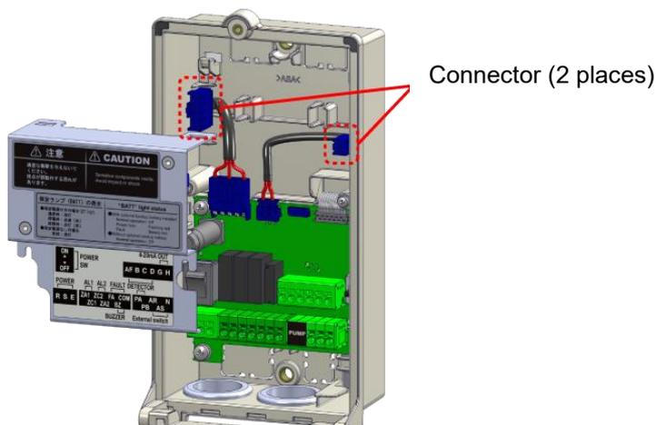
**5 Remove the two screws that attach the AC-DC power supply unit to the cover. Replace the AC-DC power supply unit with a new one. Ensure that the new AC-DC power supply unit is placed in the correct orientation.**
