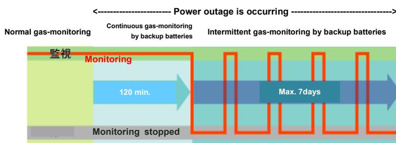
In the event of a gas alarm during the intermittent gas-monitoring mode
