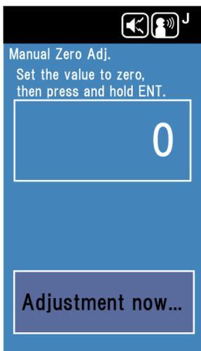
A successfully completed zero adjustment displays the following screen.
