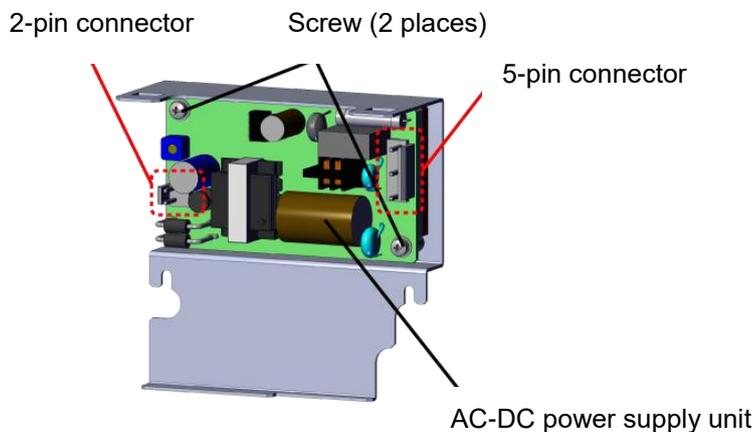
**6 Reinstall the AC-DC power supply unit by taking the reverse order 1 to 4.**
