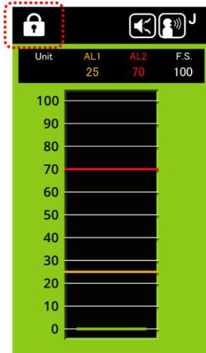
To deactivate the safety lock, simultaneously press and hold the MENU/CANCEL and ENT buttons until the lock icon disappears.
