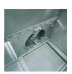
The powerful grinding mechanism with its tungsten carbide cutting teeth will handle even the most obstinate of food waste. Metal items and other residues are collected above the floor of the grinding tank in the wire sieve basket.
