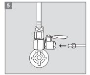
Cut the plastic tube in 2 pieces. Connect the inlet tube and tighten the tube with the cap.
