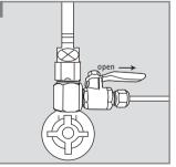
Open the diverter valve under the sink slowly. Check the whole system for water leakages.
