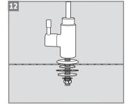
Insert the rubber washer from beneath the sink and fix the faucet in place.
