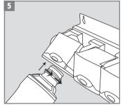
Remove the cap of the new filter and insert in the head connector. A "click" will signal that the filter cartridge is connected properly.
