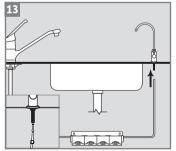
Connect the outlet tube with the drinking water faucet connector.
