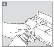
Press the push button and rotate the filter to eject.
