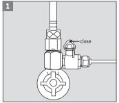
Close the diverter valve under the sink.
