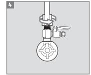
Assemble the ball valve and nipple to the water supply. Re-attach the metal hose.
