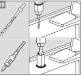
Select a proper place for the faucet. Drill a placement hole into the sink.
