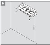
Select a proper place under the sink that has at least 25 cm (10") / 30 cm (13") from the floor to allow to insert the cartridges easily. Make holes into the wall to fix the filter adapter under the sink.
