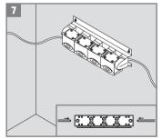
Insert the plastic tube and connect the adapter on the wall.
