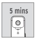
Flush the filter cartridge (by letting the filtered water flow) for at least 5 minutes after it has not been used for a long time.
