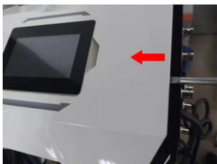
Insert the tools (screw driver) near the buckle position
