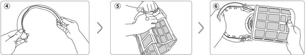
To replace the new filter basket, follow the reverse steps from the disassembly process:
