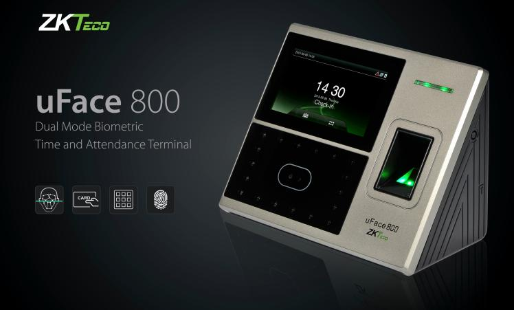
The uFace800 dual mode biometric time and attendance terminal includes both a camera for facial recognition and a fingerprint capture device for versatile and secure biometric applications.
