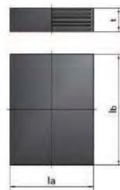
Schematic Diagram of GJZ(F4) Elastomeric Bearing
