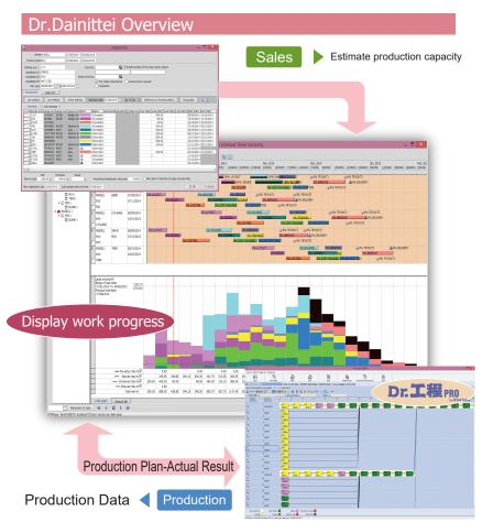
Dr.Dainittei is Schedule Management System for 3 levels: model, part and mold that display overall workload of the whole factory and synchronize with Dr.Koutei PRO to retrieve planned and actual data to calculate overall working hours.
