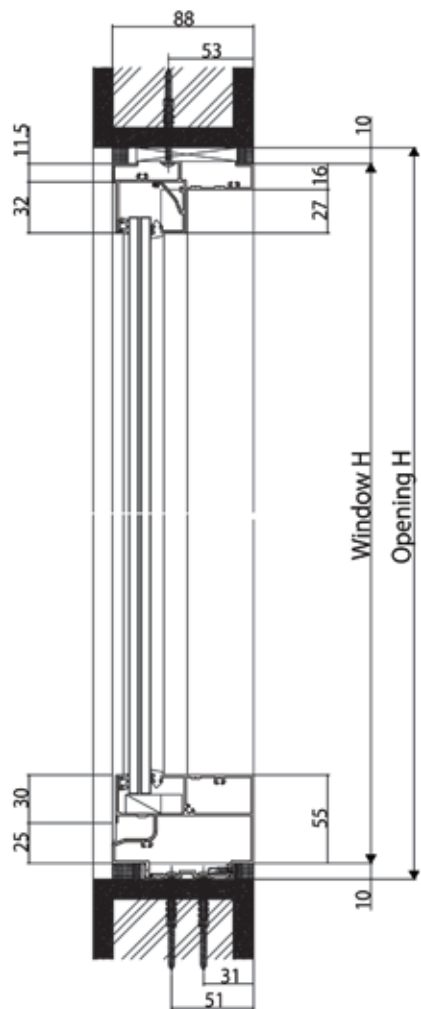
< Vertical section: Single fixed window >
