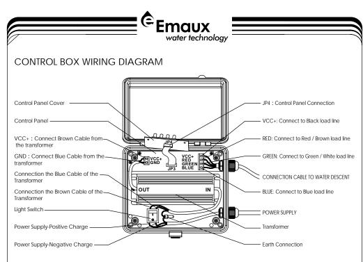
$\Delta$  Warning: load of the control box should not exceed 60W.
