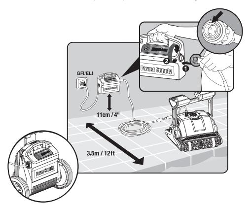
Attach the floating cable to the power supply by inserting it with the notch on the connector (1) lined up with the groove in the socket on the power supply and turning clockwise (2). Plug in the power supply and leave it in the OFF position.
