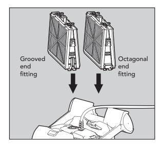
Reinstall the base frames with filters according to the diagram.
