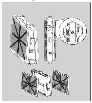
Open the clips and remove the filters.
