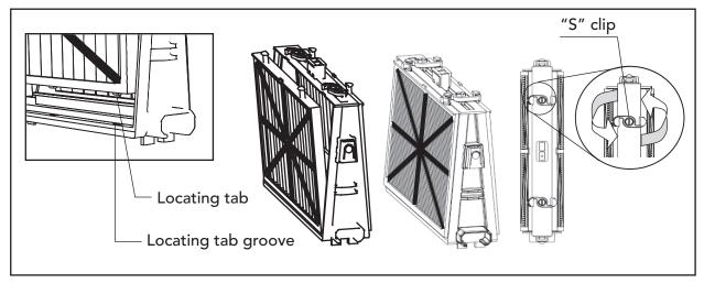
Reassembling the filter elements: Insert the locating tabs at the bottom of the filter element into their grooves on the base frame then close the "S" clip.
