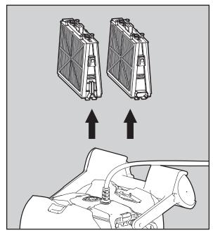
Open the filter covers and remove the cartridges from both sides of the robot.
