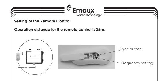
Each control box is associated with a remote control. To use a single remote to control a multiple number of control boxes, you would need to configure the Frequency at the back of the remote control. The Frequency of the Remote would then need to be synced with all the control boxes.
