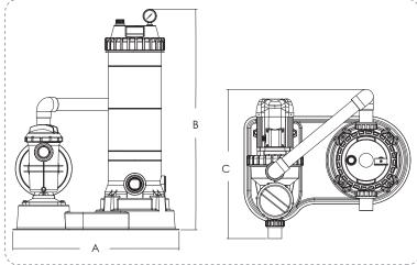
FSC Series Filtration Combo includes: 1) cartridge filter 2) cartridge filter element
