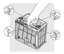
6.2.5 Assemble the filter panels according to the following order: Panel  $4 \rightarrow 3 \rightarrow 2 \rightarrow 1$ .
