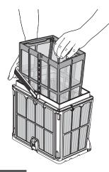
6.2.1 Hold down the handle to remove the inner net basket.
