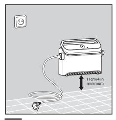
**5.1.1** Position the power supply at approximately the middle of the long side of the pool, at least at a distance of 3.5m/12ft.
