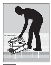
5.7.3 Place the Robotic Pool Cleaner on the side of the pool and let the water drain out.
