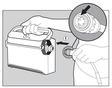
**5.1.3** Attach the floating cable to the power supply: Insert the cable with the notch on the connector (1), lined up with the groove in the socket on the power supply, and turn clockwise (2).
