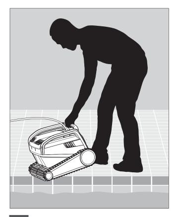
**5.2.1** Place the Robotic Pool Cleaner in the pool. Release it and let it sink to the floor of the pool. Make sure that the floating cable is free of any obstacles.
