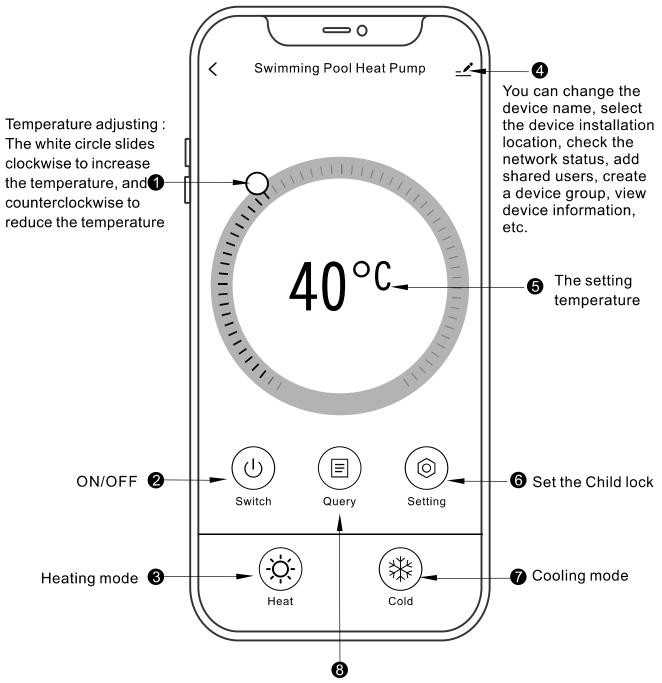
View the water inlet temperature and water outlet temperature, and the type default
