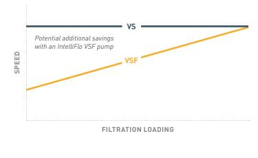
Variable Speed: RPM set high to maintain minimum flow Variable Speed and Flow: Increases speed as needed to maintain preset flow
