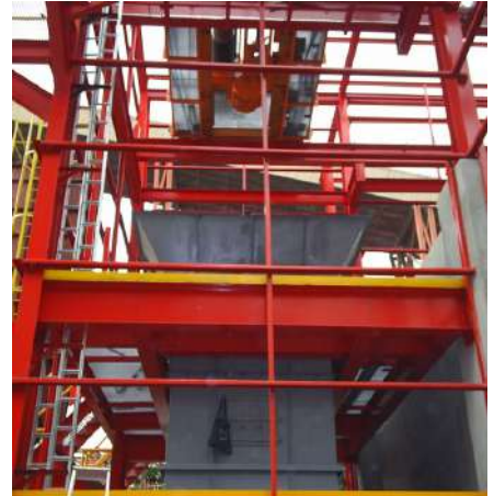
Fine material extractor: To load fine solid AFR with accurate dosage.
