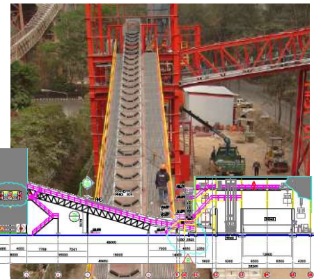
Fine material extractor: To load fine solid AFR with accurate dosage.
