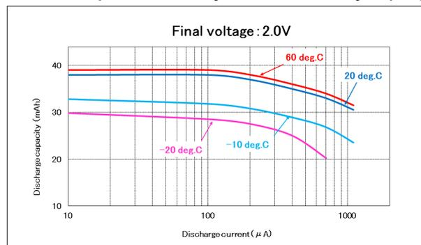
\* Nominal capacity indicates duration until the voltage drops down to 2.0V when discharged at a nominal discharge current at 20 deg. C.
