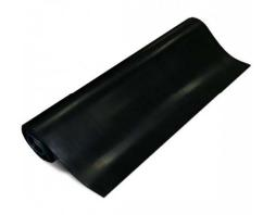
Montero NBR Rubber Gasket Style 9210 is premium grade nitrile, 60 to 85 duro, generally resistance to most hydrocarbon, fats, oils, greases, hydraulic fluids, chemicals and solvents,
