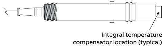
Figure 1 Temperature compensator location
