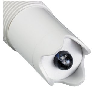
Low temperature (LT) glass with notched body
