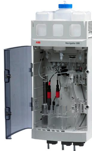
The Navigator 550 sodium wet-section has been designed to be used in conjunction with the Navigator 540 transmitter either alone or in combination with other Navigator 550 wet-sections.
