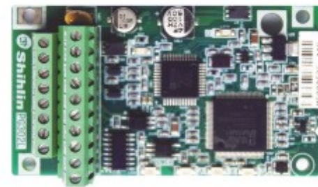
PG302L Speed feedback board (supports Resolver signal)
