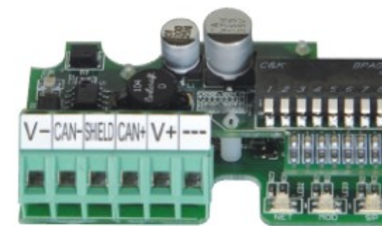
SE2-DN01 Device-Net communication board
