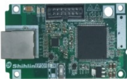
EP301 Ethernet communication expansion board
