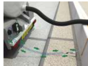
Continuous Ground Loop Monitoring check
