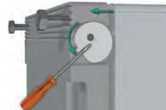
Excenter disk for easy opening
