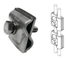
Universal Connector is made of Stainless Steel. There are two types of connecting process cross joint and parallel joint. The contact resistance shall be less than 1 m $\Omega$ , as well as the connected conductors tensile force s hall be more than 900 N
